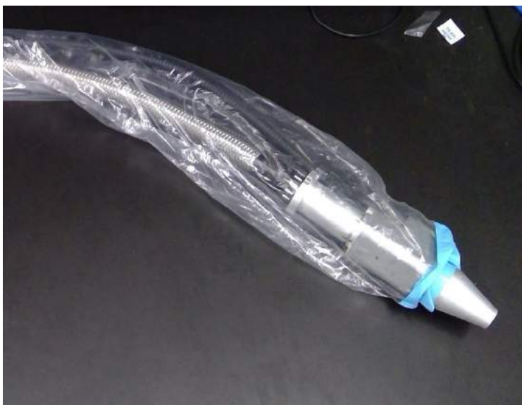
Figure 4: Sterile drape wrapping the probe and the imaging bundles
